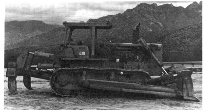
Bulldozer. Note the smoke stack (exhaust pipe).
